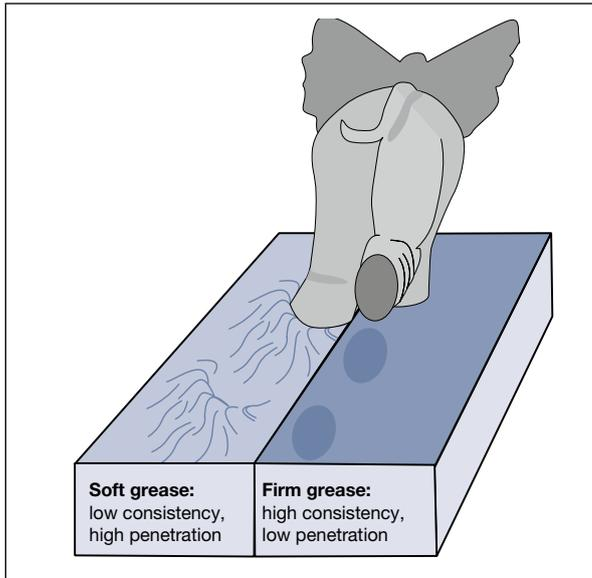
Consistency of a lubricating grease
