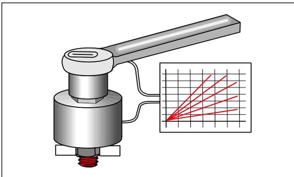
Measuring the thread friction
